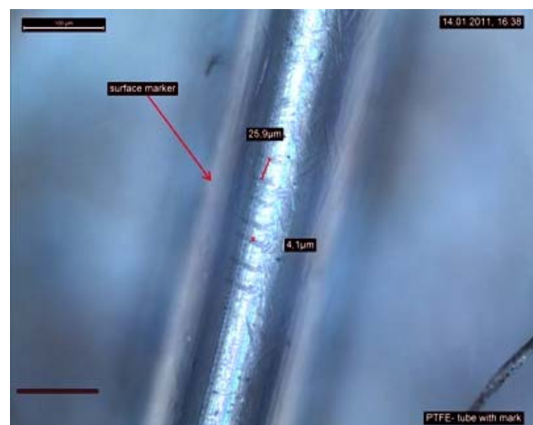
PTFE microtube, Ø 400µm – the outer surface marked with a micro-code periodic size of 4µm regular shaped lines.
