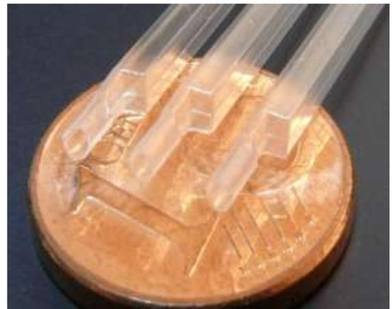
**Demonstrator products made from polymer micro-tubes**
